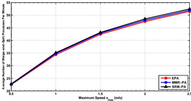
Fig. 7. Average Number of Merge-and-Split Processes Under the Proposed Distributed Algorithm - Network Density = 0.005 Nodes/Unit Square Area
