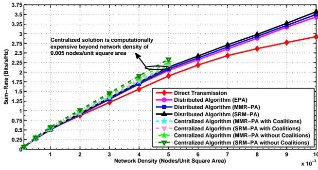
Fig. 2. Network Sum-Rate of Different Power Allocation Criteria
