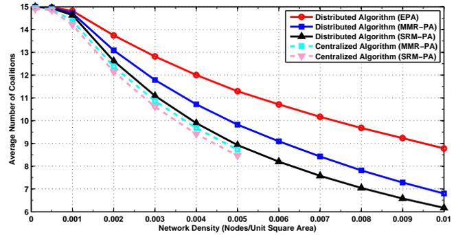
Fig. 4. Average Number of Coalitions of Distributed and Centralized Algorithms
