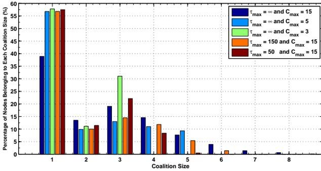
Fig. 11. Percentage of Nodes Belonging to Each Coalition Size Under the Proposed Distributed Algorithm - EPA Criterion with Time-Index and Coalition Size Constraints - Network Density = 0.01 Nodes/Unit Square Area
