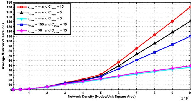
Fig. 10. Average Number of Iterations Under the Proposed Distributed Algorithm - EPA Criterion with Time-Index and Coalition Size Constraints
