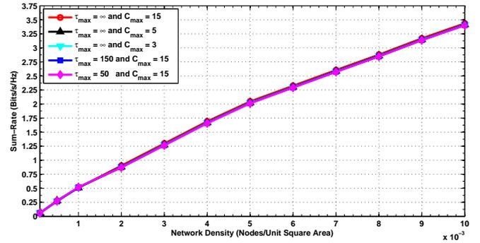
Fig. 9. Network Sum-Rate Under the Proposed Distributed Algorithm - EPA Criterion with Time-Index and Coalition Size Constraints
