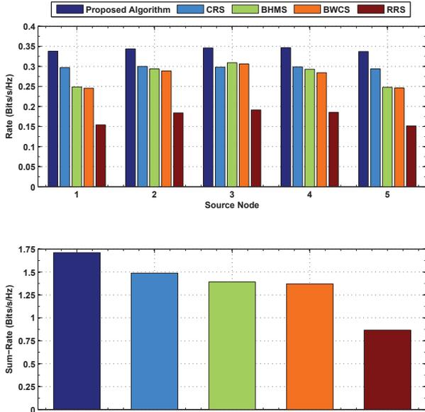
Fig. 5. Achievable Rate of Each Source Node and Network Sum-Rate Under Different Relay Selection Schemes vs. Distributed Relay Selection Algorithm - Scenario 1 - ERP Allocation Scheme
